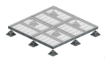
**Total Frame Capacity** Distributed Deadload 22,400 lbs Distributed Windload 5,980 lbs Channel Capacity (Critical Load Point) Concentrated Deadload 4,000 lbs Concentrated Uplift 4,000 lbs
